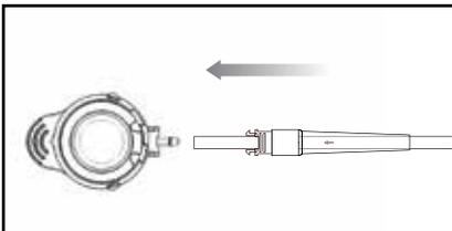
**Figure 2. Tubing alignment with Access Port's outlet barb**
