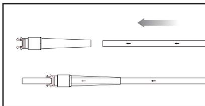
**Figure 1. Strain Relief and end of tubing alignment**
